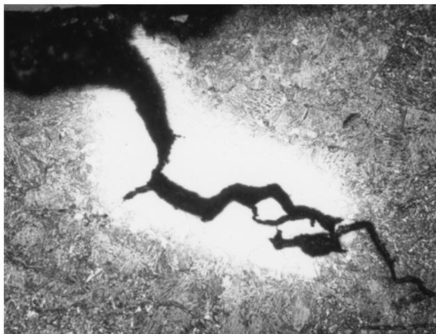
**Figure 6.5f.** Sword 4. A pronounced crack starting on the surface of the edge in the left part of the section. Decarburisation has occurred around the crack due to long heating time during forging. (100x).
