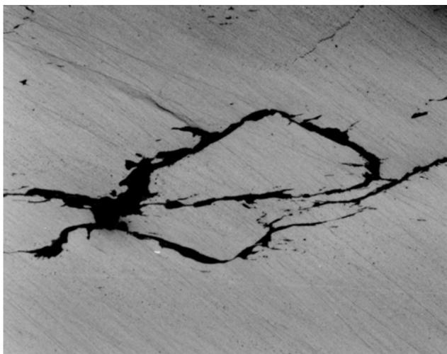
Figure 6.19b. Sword 18. Unetched. A few bent hammer scale structures in the left part of the section indicate that pieces of iron were folded and forged together. (50x).
