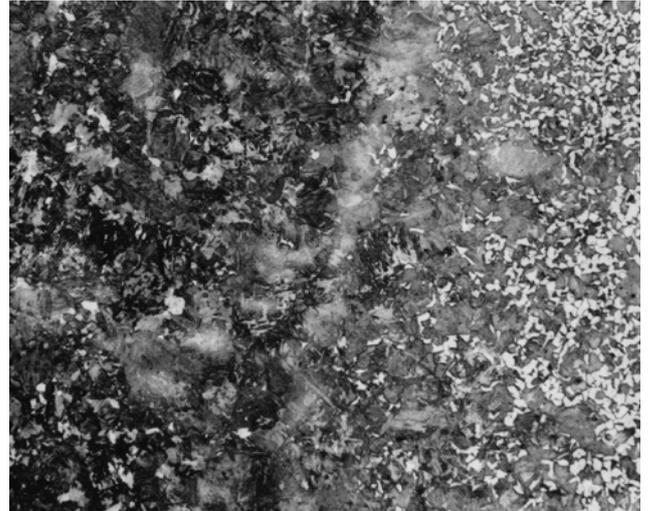
**Figure 6.10e.** Sword 9. Some diffusion of carbon from the carbon-rich dark edge (dark part) across the welding seam. Left edge shown. (100x).
